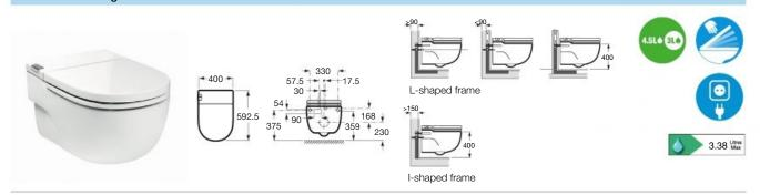
Wall-hung WC with integrated cistern and 4.5/3 litre dual-flush. Soft-close seat and cover included. Requires electricity for the air pump used in the flushing process. Works on mains pressure only. Installation videos and information (including pre-installation) are available at www.uk.roca.com
