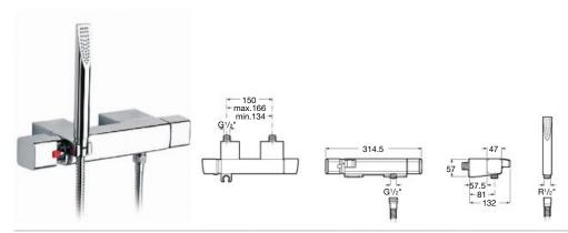
**5A1350C00** Wall-mounted thermostatic shower mixer with handset, 1.7m flexible shower, integrated holder and 1/2" water connection
