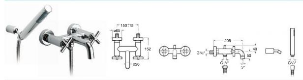
5A0143C00 Wall-mounted bath-shower mixer with automatic diverter with retention, 1.75m flexible shower hose, handset, swivel wall bracket and 1/2" water connection
