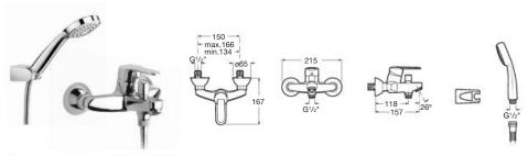
5A0125C02 Wall-mounted bath-shower mixer with automatic diverter with retention, 1.7m flexible shower hose, Natura handset, swivel wall bracket and 1/2" water connection
