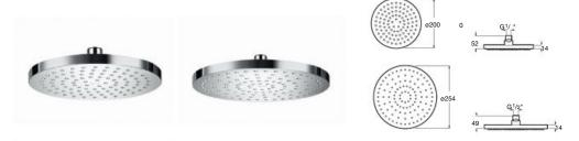
Circular high-flow shower head with pivot connection and 1/2" water connection. Can be mounted on wall or ceiling with optional fixing kits. Chrome plated ABS. Features EasyClean nozzles to help prevent limescale build-up.
