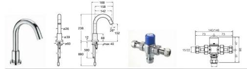
Electronic monobloc basin faucet (single water supply) with flexible supply hose and integrated spout sensor. Powered by 4 AA alkaline batteries (1.5V LRG).
