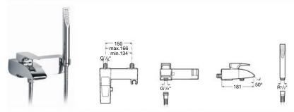
5A0150C00 Wall-mounted bath-shower mixer with automatic diverter with retention, 1.7m flexible shower hose, handset, integrated holder and 1/2" water
