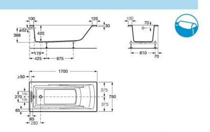
1700 x 750 Acrylic bath including headrest (code 24F061000). Supplied with adjustable legs. Capacity: 195 litres up to overflow 248162000
