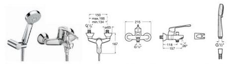
**5A0123C02** Wall-mounted bath and shower mixer with automatic diverter with retention, 1.7m flexible shower hose, handset and swivel wall bracket
