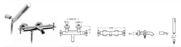
5A1143C00 Wall-mounted thermostatic bath-shower mixer with diverter-flow regulator, 1.7m flexible shower hose, handset, swivel wall bracket and 1/2" Optional: D50010022 Easy Fix Kit (for installing bar shower valve to pipework) D50010009 Pillars (allowing product to be deck-mounted)
