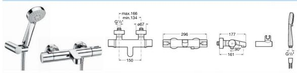
**5A1146C02** Wall-mounted thermostatic bath-shower mixer with diverter-flow regulator, 1.7m flexible shower hose, Stella 80/3 handset, swivel wall bracket and 1/2" water connection
