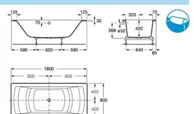
8 1800 x 800 Double-ended acrylic bath including 2 headrests (code 24F061000). Supplied with adjustable legs. Capacity: 223 litres up to overflow 248163000
