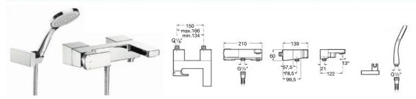
5A0101C00 Wall-mounted bath-shower mixer with automatic diverter with retention, 1.7m flexible shower hose, L90 handset, swivel wall bracket and 1/2" water connection
