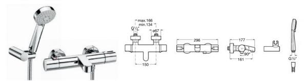
5A1146C02 Wall-mounted thermostatic bath-shower mixer with diverter-flow regulator, 1.7m flexible shower hose, Stella 80/3 handset, swivel wall bracket and 1/2" water connection
