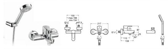
5A0109C02 Wall-mounted bath-shower mixer with automatic diverter with retention, handset, 1.70 m flexible hose, Stella 80/1 handset, swivel wall-bracket and 1/2" water connection Optional:
