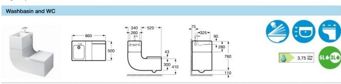
hoses. Features Roca's water reuse technology (water from the basin is filtered and reused to flush the WC). Installation videos and information (including pre-installation) are available at www.uk.roca.com
