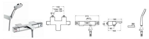
5A1101C00 Wall-mounted thermostatic bath-shower mixer with 1.7m flexible shower hose, L90 handset, swivel wall bracket and 1/2" water connection D50010022 Easy Fix Kit (for installing bar shower valve to pipework) D50010009 Pillars (allowing product to be deck-mounted)
