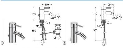
5A6011C00 ① Monobloc bidet mixer with swivel flow regulator, pop-up waste and flexible supply hoses
