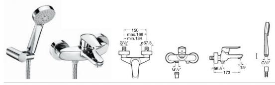
5A0127C02 Wall-mounted bath-shower mixer with automatic diverter with retention, 1.7m flexible shower hose, Stella 80/3 handset, swivel wall bracket and 1/2" water connection
