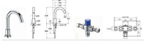
**5A4243C00** Electronic monobloc basin faucet (single water supply) with flexible supply hose and integrated spout sensor. Powered by 4 AA alkaline batteries (1.5V LRG).
