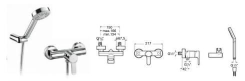
5A2009C02 Wall-mounted shower mixer with 1.5m flexible shower hose, Stella 80/1 handset, swivel wall bracket and 1/2" water connection D50010022 Easy Fix Kit (for installing bar shower valve to pipework)
