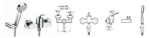
5A2046C02 Wall-mounted shower mixer with 1.5m flexible shower hose, Stella 80/3 handset, swivel wall bracket and 1/2" water connection
