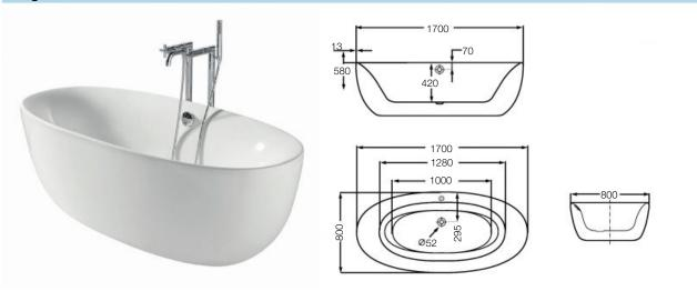
248313000 One-piece acrylic bath with integrated panel and pop-up waste. Supplied with adjustable legs. For freestanding installation. Capacity: 175 litres up to overflow
