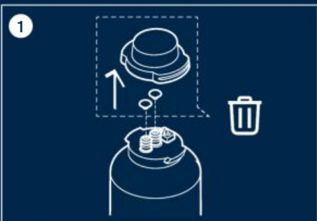
1. Rotate 90 degrees the old filter to disassemble.
