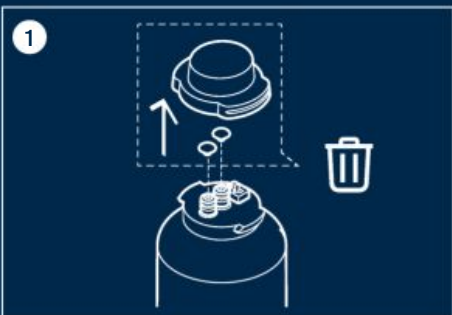
1. Rotate 90 degrees the old filter to disassemble.
