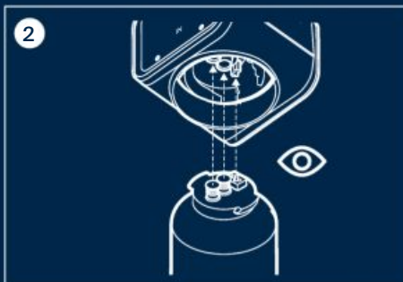
2. Remove the lid from new filter and assemble it to the head (rotating 90 degrees).
