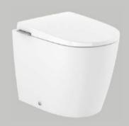
Back to wall hydraulic toilet with integrated tank of dual flush 4,5/3L. Includes Roca Rimless\* Vortex, soft-closing seat and cover and Supraglaze\* glazing. No need for built-in cisterns. Internal hydraulic water supply connection.
