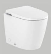
Back to wall hydraulic toilet with integrated tank of dual flush 4,5/3L. Includes Roca Rimless\* Vortex, soft-closing seat and cover and Supraglaze\* glazing. No need for built-in cisterns. External hydraulic water supply connection.
